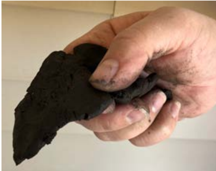
Figure 1. Determining clay content in soil via the ribbon test. The ribbon length indicates the soil is fine-textured.
