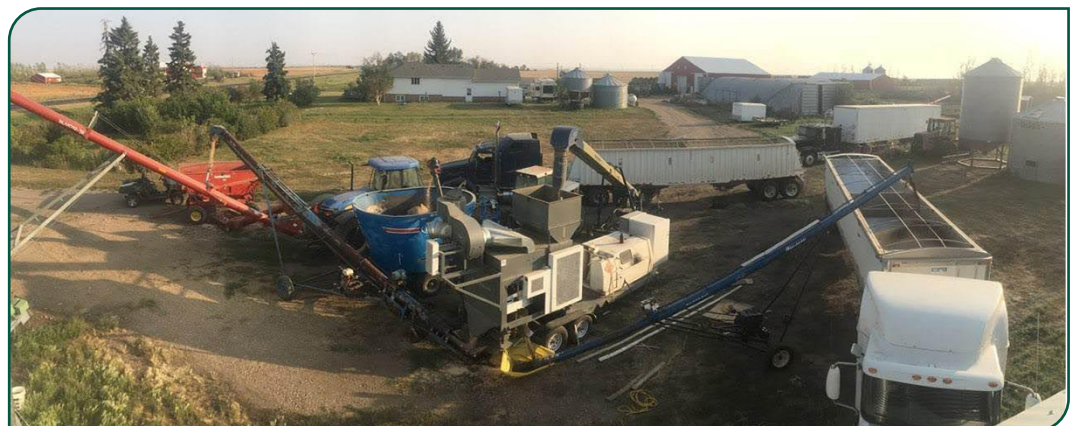
Figure 3. Separating and cleaning pea-canola intercrop using a portable seed cleaning unit. Mixed grain enters the cleaner via the auger in the middle, clean canola exits via the blue auger on the right, clean pea exits via the brown auger on the left, and screenings are collected in the round blue tub behind the cleaning unit. [M. Jacobs]
