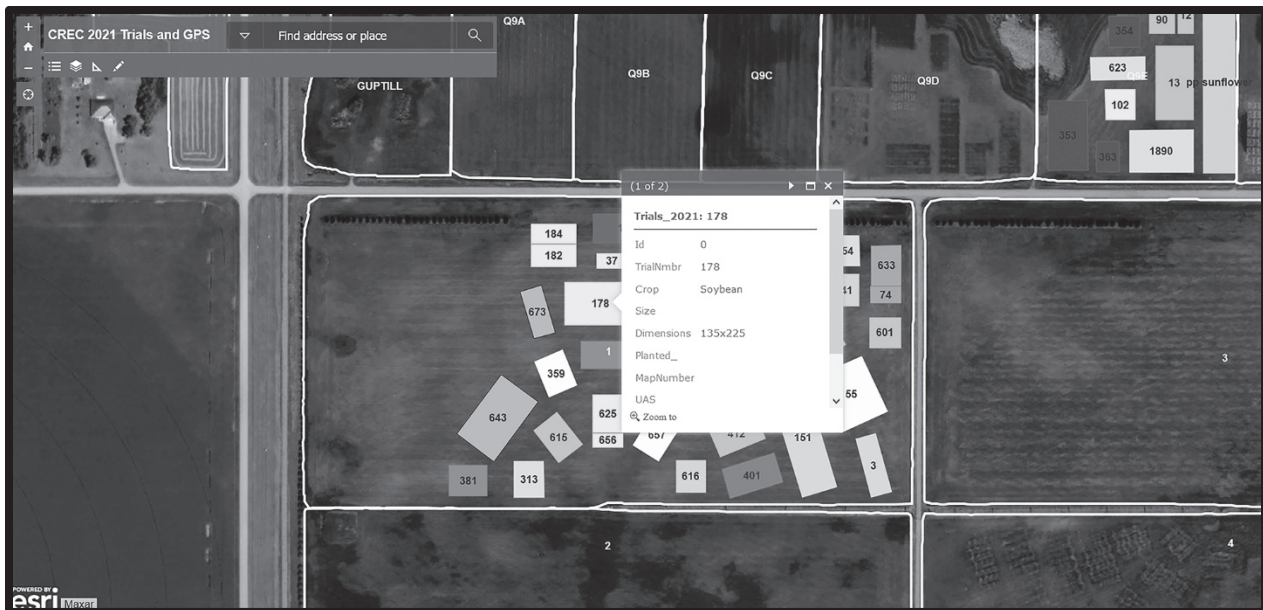
Figure 3. After zooming in, attribute information can be readily obtained by clicking on the trial. Conversely, the search bar in the top left will simultaneously zoom to the plot while opening the attribute window.
