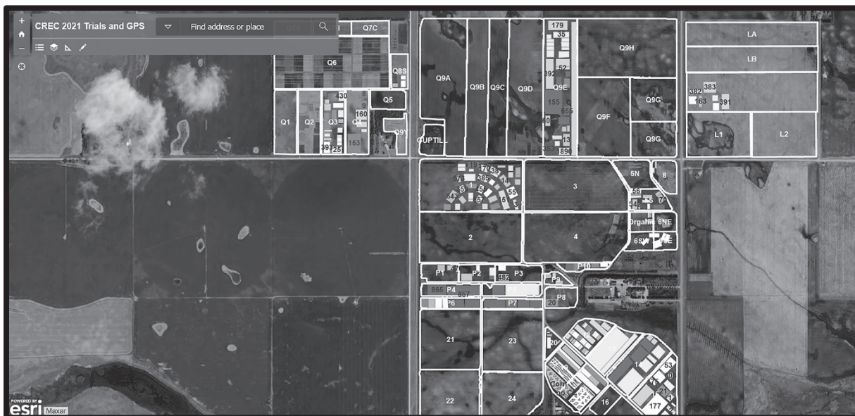
Figure 2. The web-based implementation allows CREC staff to search for trials using the embedded attribute search functionality or identify trials by simply clicking on the polygon to retrieve the associated attributes. Additional tools for measurements and toggling the legend are also included.
