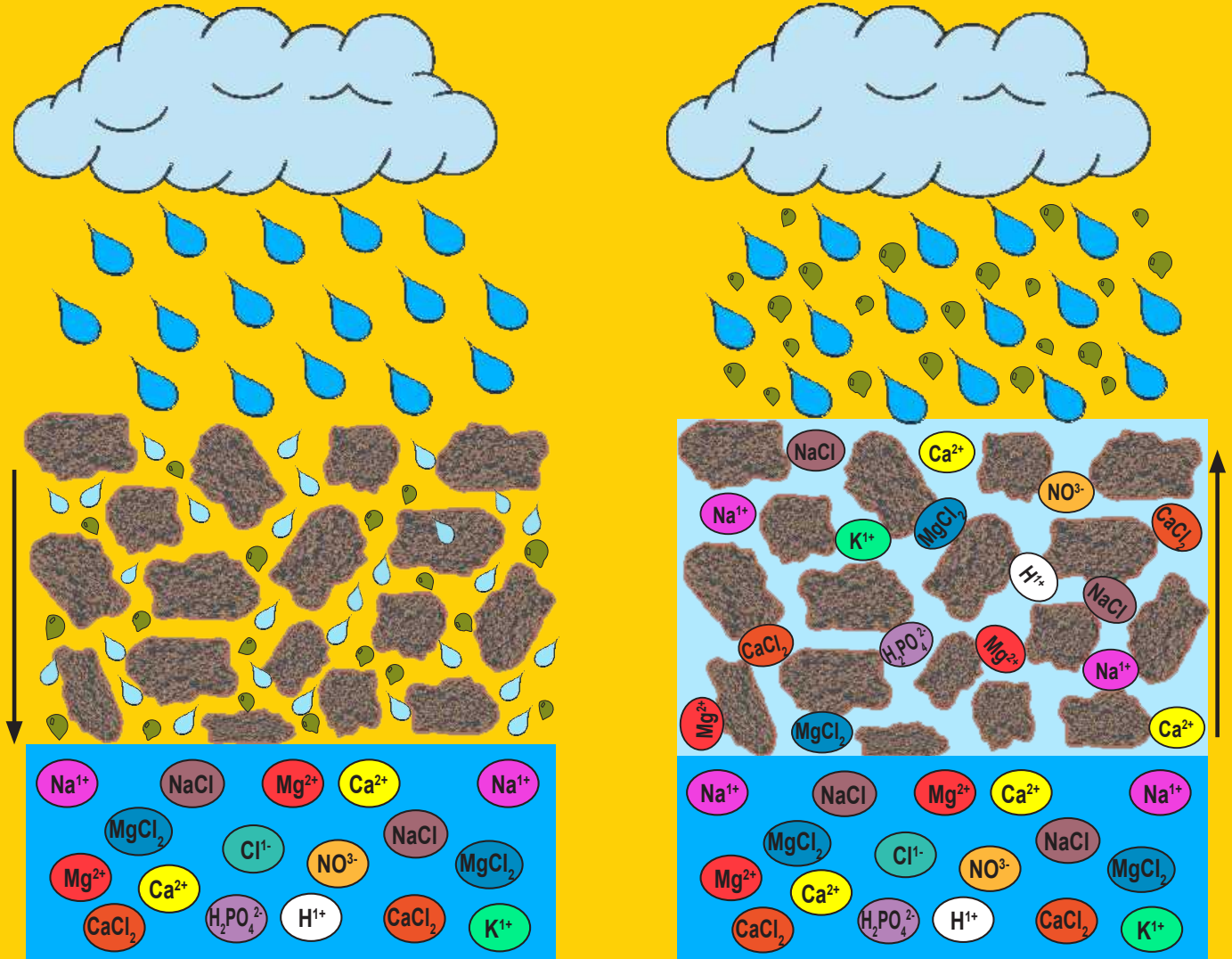
Figure 6. A well-drained soil with low groundwater level (left) versus a saturated soil with very shallow groundwater level on the right.
