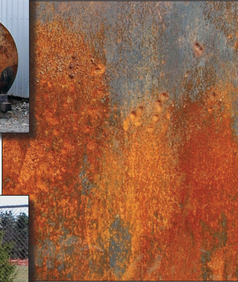
Above and right: These underground fuel tanks are being reused for aboveground storage. Notice the extreme corrosion in the right-hand photo. Tanks previously used underground should never be reused for aboveground fuel storage.
