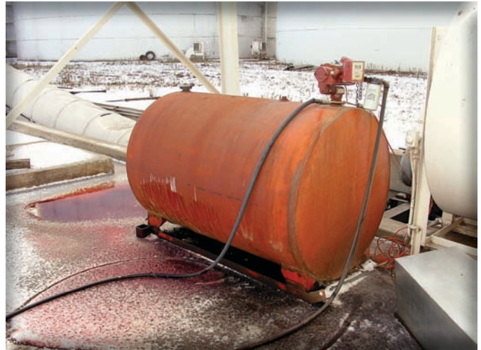
Automatic nozzles do not always shut off. Require anyone fueling equipment to remain at the fuel nozzle.
