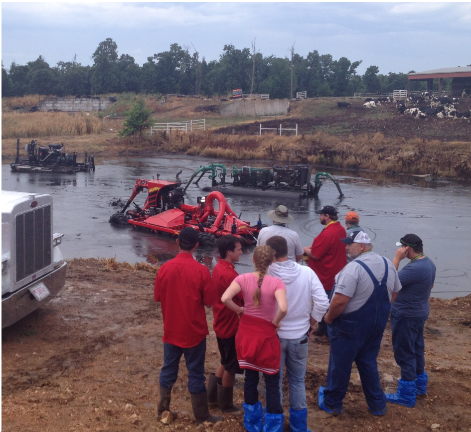
Various liquid manure agitators homogenize a lagoon at the North American Manure Expo near Springfield, MO.
