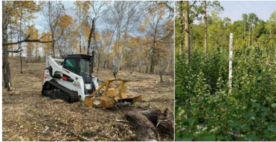
A forestry brush cutter is used to clear old decadent aspen; giving way to lush regrowth
