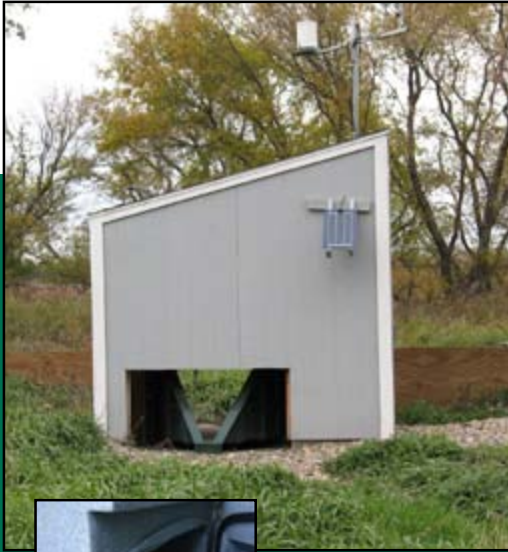
Pictured is an example of a Discovery Farms gaging station. Runoff water passes through the flume below the shed; samples are collected and bottled inside automatically for analysis by U.S. Geological Survey officials.
