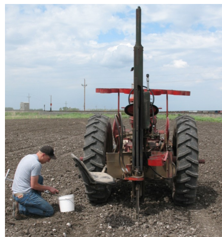
Soil sampling with a 12inch hand probe and 4 feet Guidings probe
