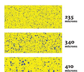
These are examples of spot cards measured by WRK Droplet Scan. The application rate was 5 gallons/acre.
