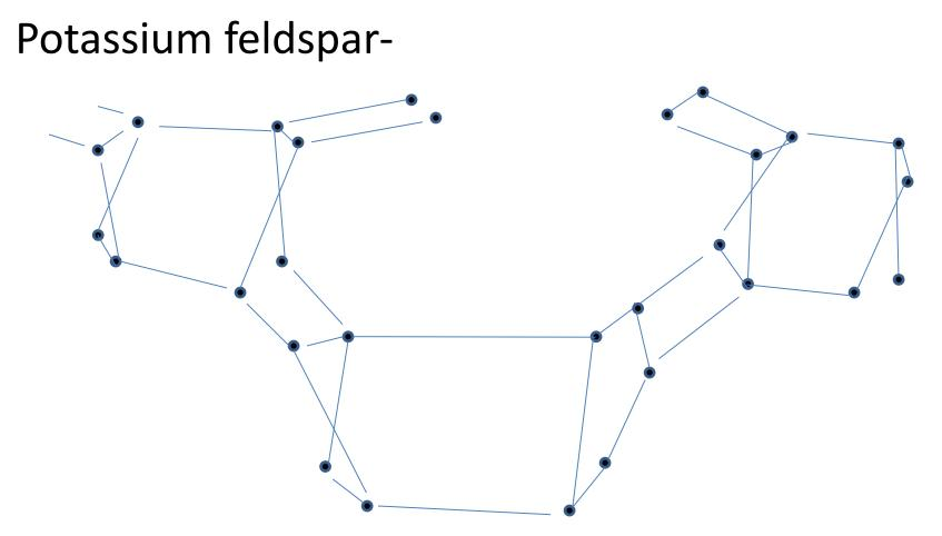
3-D framework of SiO4 and Al2O3 tetrahedrals isomorphous substitution of Al for Si ~ ¼ of the time results in significant negative (-) charge. Potassium within the open spaces helps balance charge.
