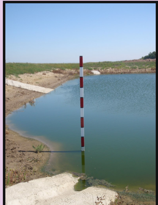
Monitoring pond levels and land-applying effluent before a pond is full prevents the containment pond from overflowing.
