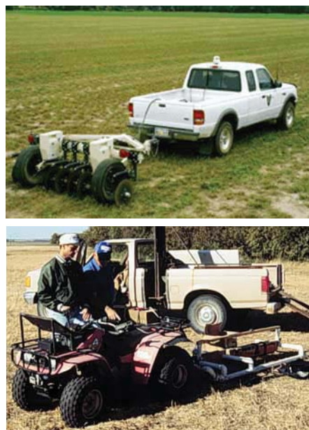
Figure 6. Veris conductivity sensor (top), EM-38 in use. (Norm Procnow and Hal Weiser, USDA-NRCS, Jamestown, N.D.)
