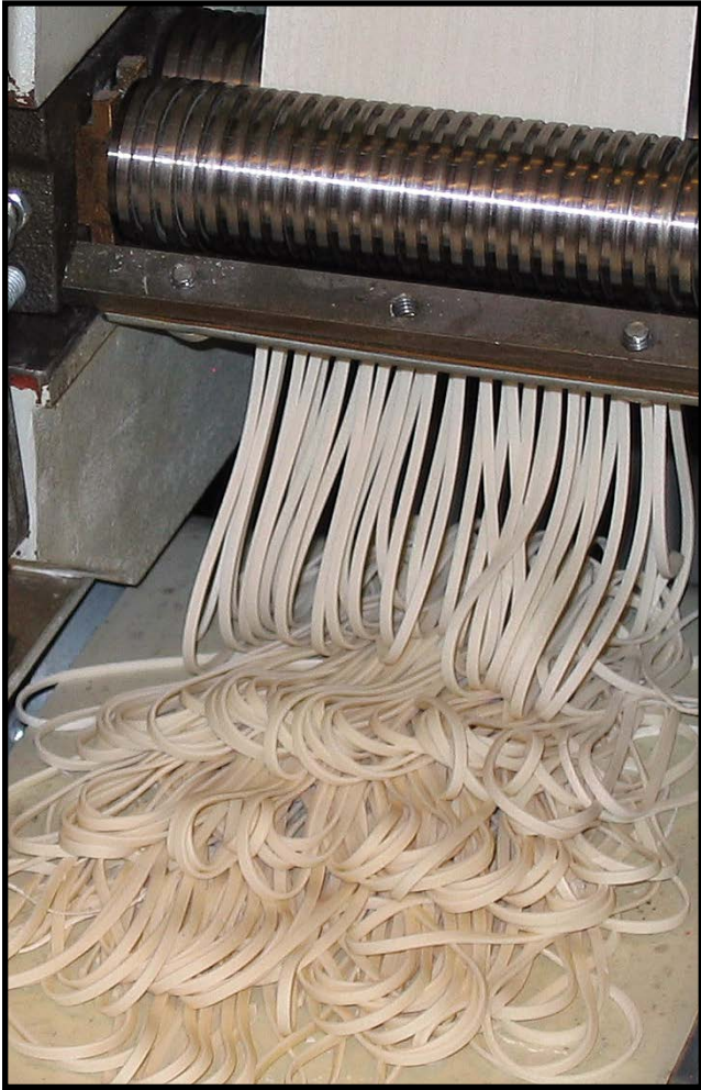
Figure 3. Unlike pasta products, which are extruded, Asian noodles are cut from sheets of dough.
