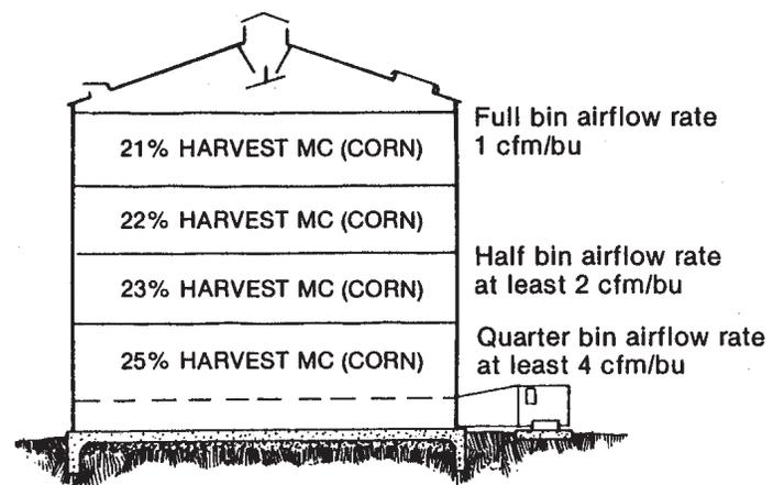
**Figure 13. Example of layer drying. The higher airflow rates on a per bushel basis early in the filling permit a higher initial moisture content to be loaded.**
