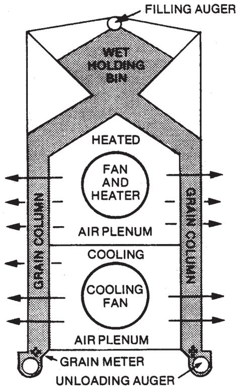
Figure 1. Cross-flow dryer with forced-air drying and cooling.
