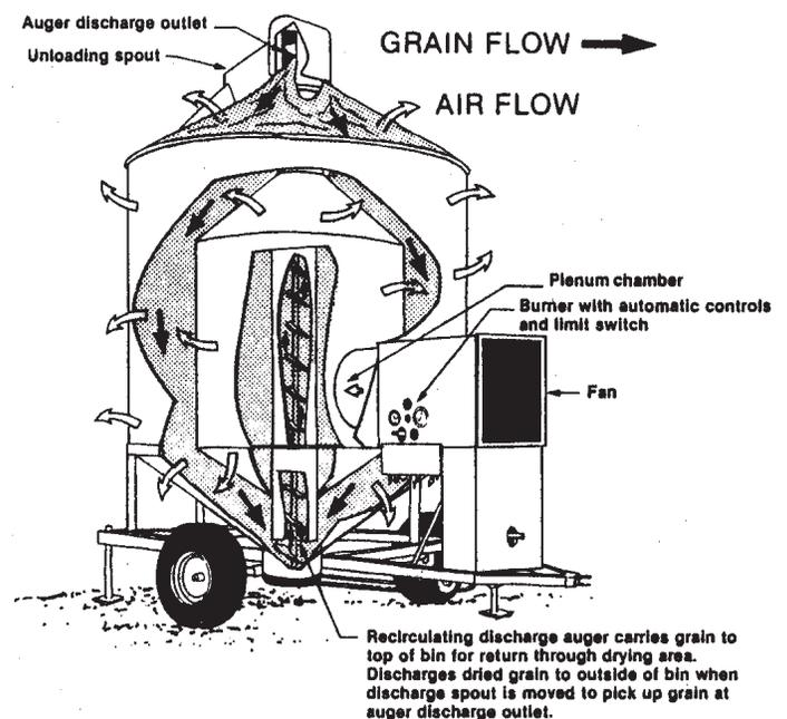
Figure 3. Recirculating batch dryer.
