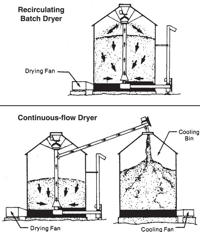
**Figure 10. Grain recirculators convert a bin dryer to a high speed recirculating batch or continuous flow dryer.**
