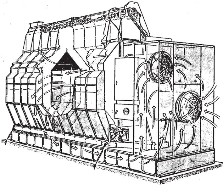
**Figure 7. Exhaust air recirculation to improve energy efficiency.**
