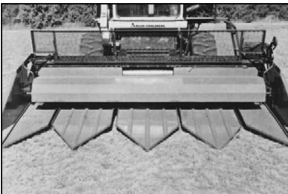
■ Figure 121. Catch pans in wide 37 inch pans spaced on 36 inch centers. (V. Hofman)
