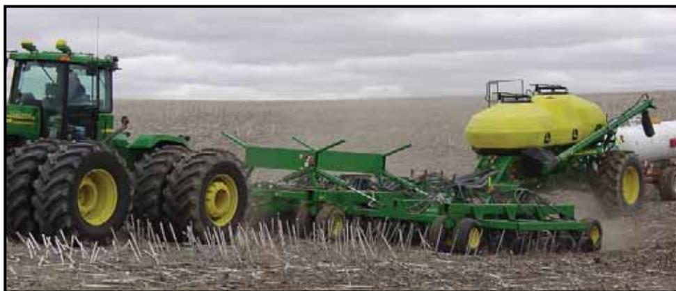
■ Figure 13. This one-pass seeding operation is seeding directly into wheat stubble. Anhydrous ammonia and seed are banded through special openers. Glyphosate and sulfentrazone were applied three days prior to seeding. (Roger Ashley)
