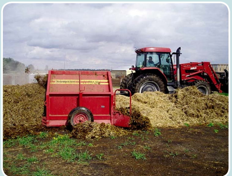
Figure 8. A pull-type compost turner that is turning windrowed bedded feedlot manure for the first time.
