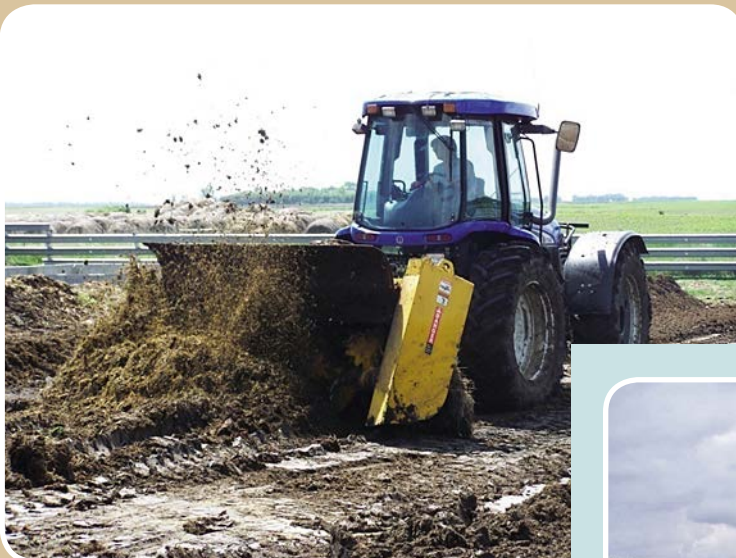
Figure 7. Front-mount composter. This compost turner cleans pens, windrows and turns the pile in the same pass.
