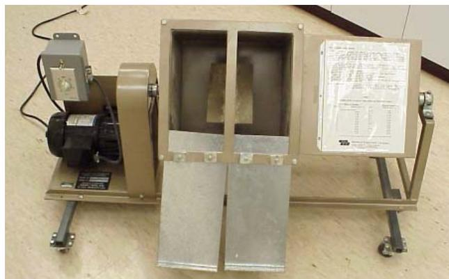
**Figure 1. Tumbler used to test pellet durability.**
