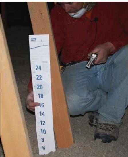
Figure 1. Measuring attic insulation thickness.
