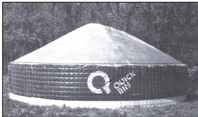
Figure 7. Sidewalls on this type of storage are reinforced with wire mesh and used to support walls 4 feet to 6 feet high. Covers can be reinforced plastic sheeting. Bins are filled with augers.
