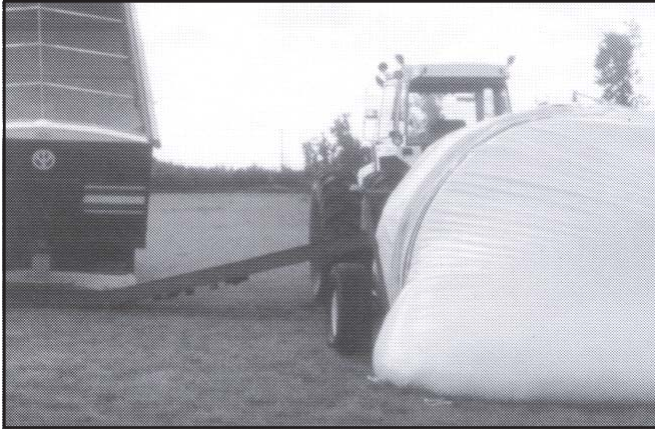
Figure 8. Round tubes of plastic about 8 feet in diameter have been developed for silage storage. Limited experience with these for dry grain storage has been satisfactory. Consult with manufacturers for their up-to-date experience. Special filling equipment or technique will be needed.
