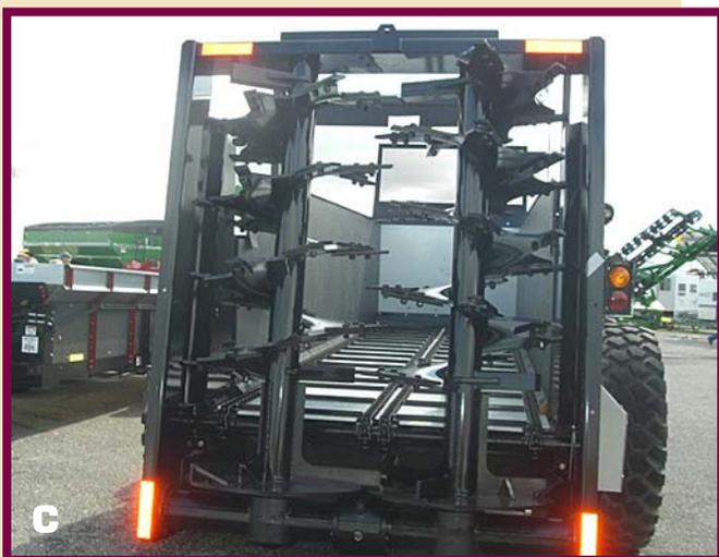
**Figure 2. Manure spreader configurations: a) spinner spreader, (b) double horizontal beater and c) double vertical beater**
