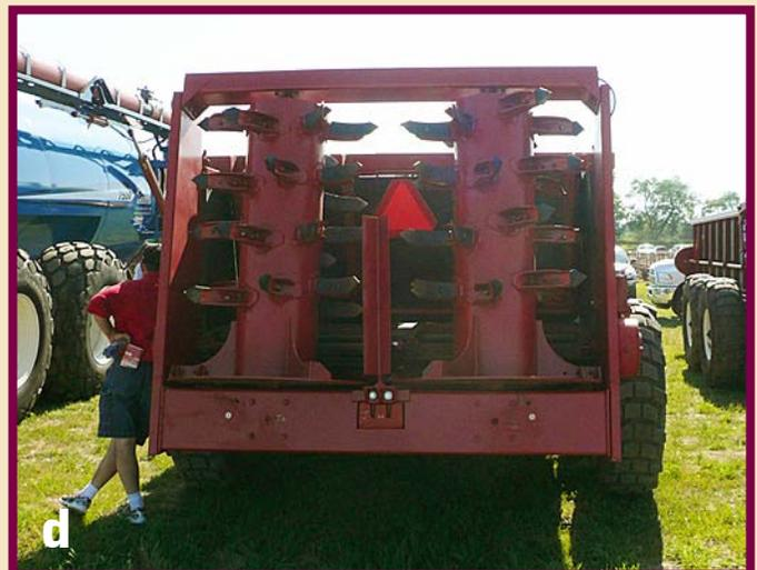
**Figure 3. Rear-delivery double-beater spreader configurations: (a) Double vertical beaters with lower spinner disks, (b) Double vertical beaters with lower spinner disks and hydraulic push manure spreader, (c) Chisel teeth horizontal beaters, (d) Chisel teeth vertical beaters** (Shafiqur Rahman, NDSU)
