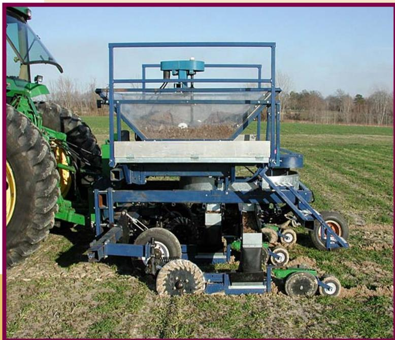
**Figure 4. Side view of a prototype of the subsurface band applicator implement for poultry litter developed by USDA-ARS at Auburn, Ala.** (Source: Thomas Way, USDA-ARS).
