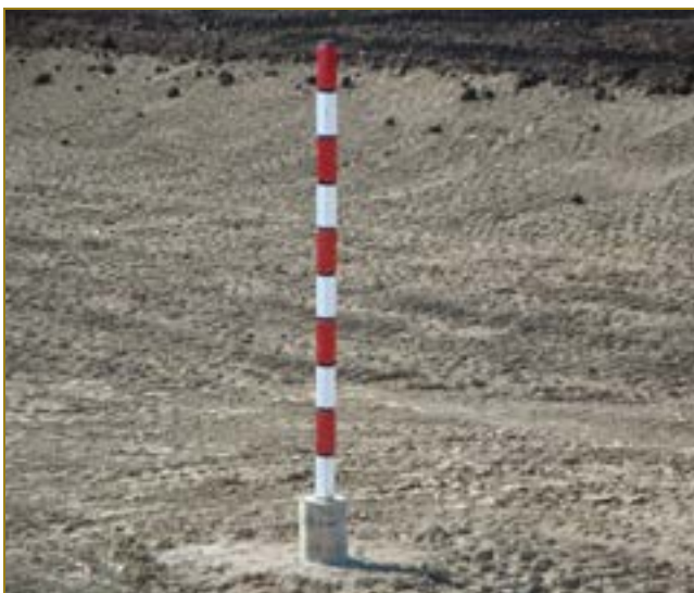
Fig. 4. Installation of pond marker when the pond is empty or under construction (photos courtesy of K2S Engineering)
