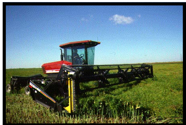
Figure 8. Swather equipped with vertical cutter bar.
