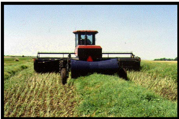
Figure 9. Rolling a canola swath.
