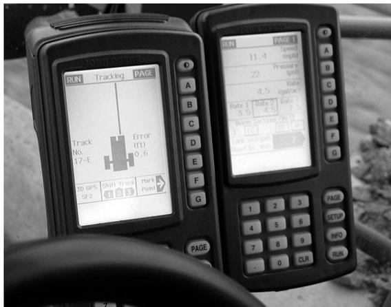
GPS receivers designed for guidance can be used in conjunction with a yield monitor or for other positioning equipment.
