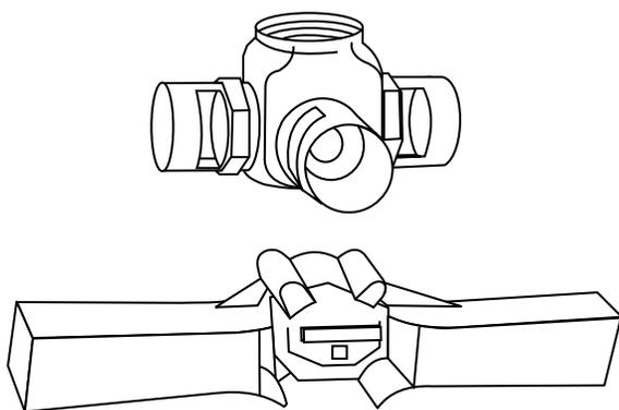
**Figure 9. Sparge tube.**
