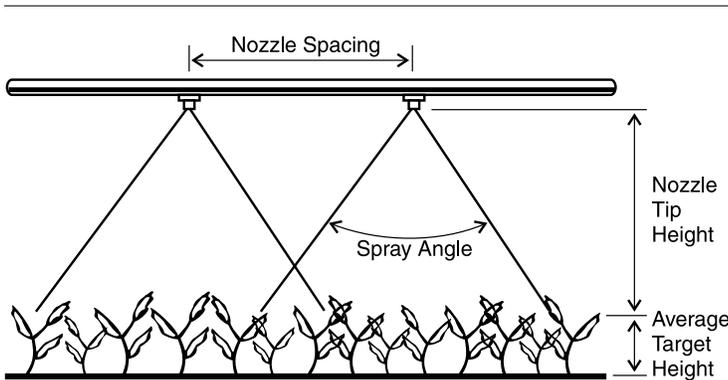
Figure 18. Discharge pattern of an “Even” spray nozzle.
