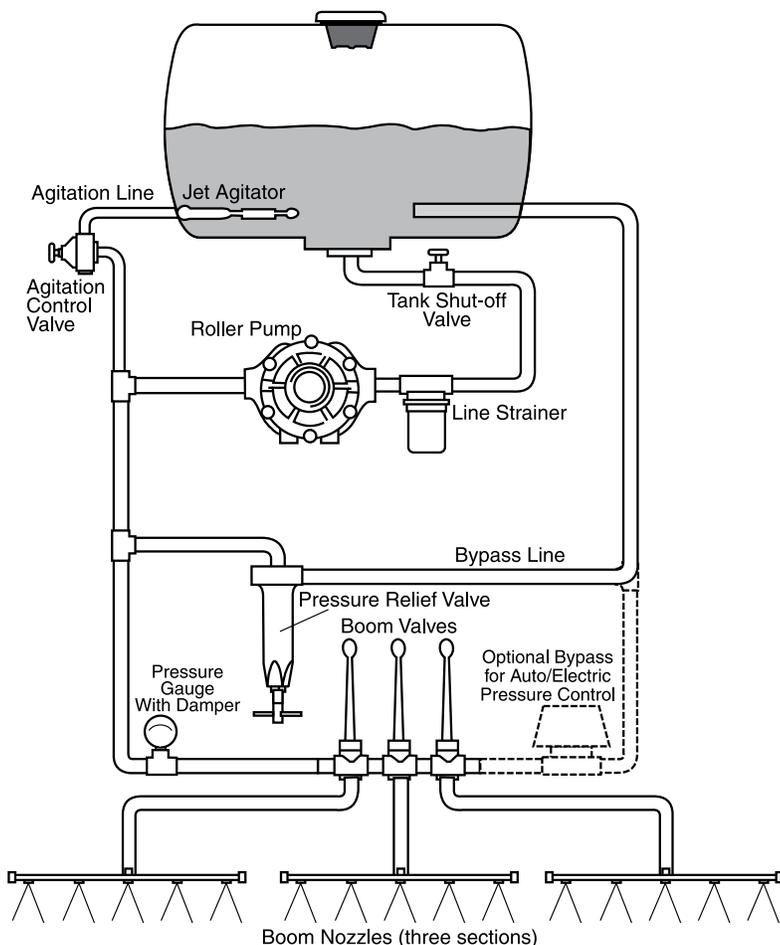
**Figure 5. Pressure relief valve.**
