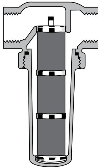
**Figure 11. Self-cleaning line strainer.**
