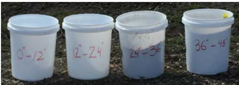
Figure 6. A 4-foot-deep sample is being separated in 12-inch increments.
