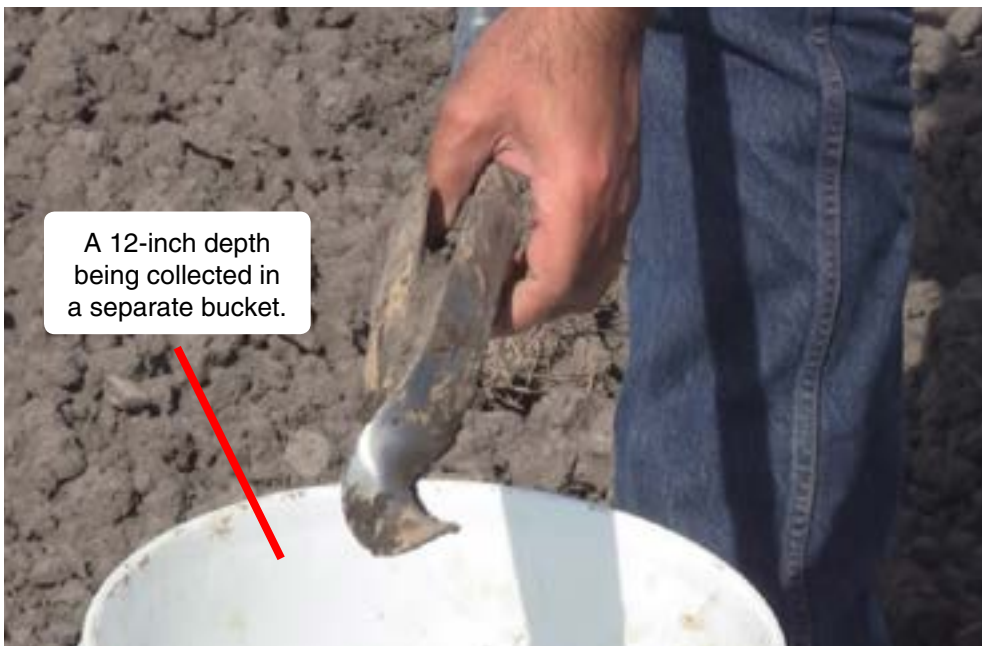
Figure 5. Soil depth is being separated in 12-inch increments.
