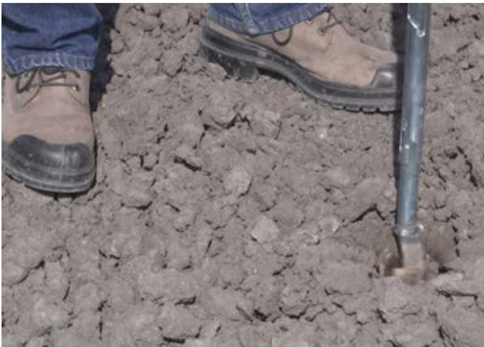
Figure 4. A soil core is being taken from a saline-sodic zone with a hand-held auger.
