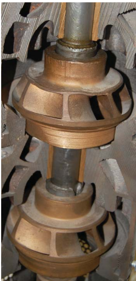
Figure 5. Cutaway view of two enclosed impellers within their pump bowls.
