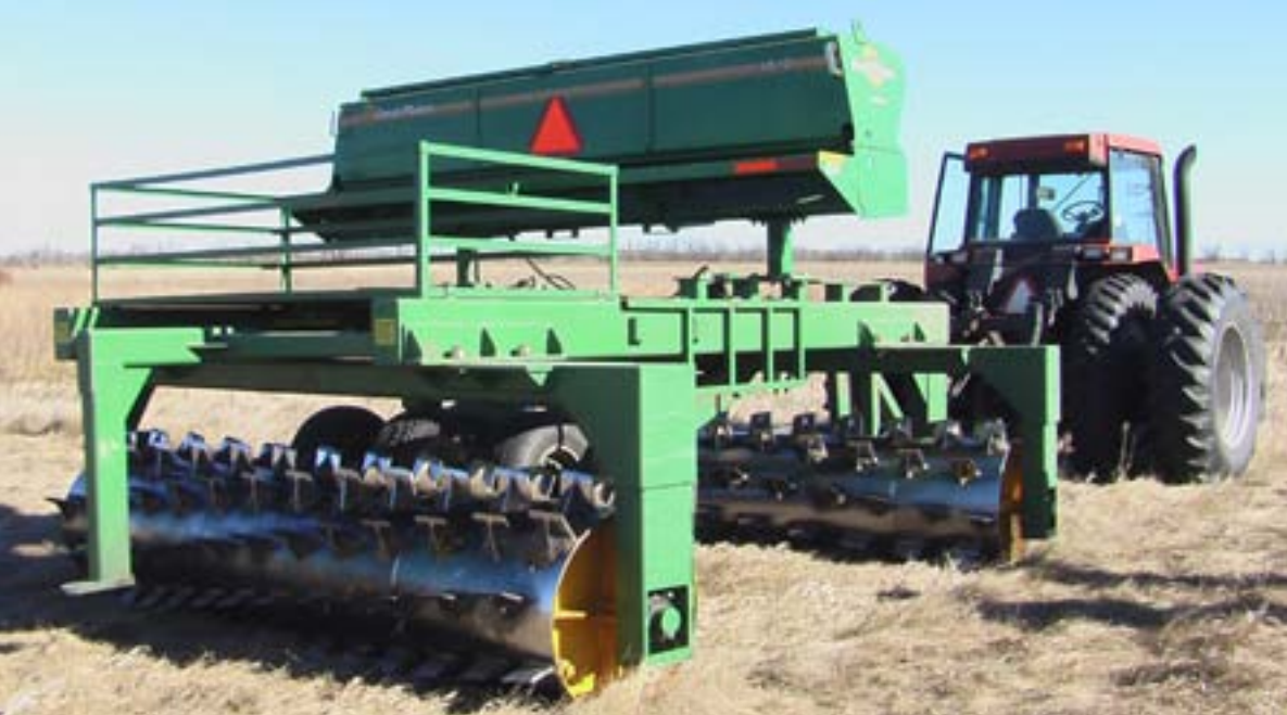
Aerator rollers can be used to cut residues into manageable lengths and flatten animal mounds prior to no-till planting.
