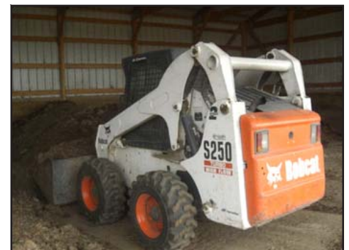
Figure 1. Composting bins and compost pile preparation using a skid-steer loader.
