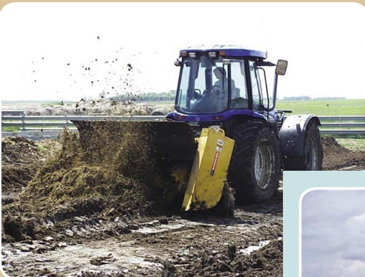
Figure 7. Front-mount composter. This compost turner cleans pens, windrows and turns the pile in the same pass.
