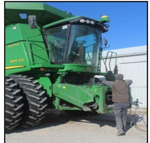
Figure 4. Raise the feeder house and lock it into place
