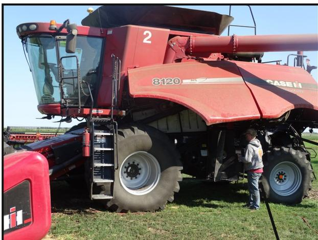
*Figure 9 (left): Open up the shields to used compressed air to clean underneath, and the exterior portions of the combine shields.*
