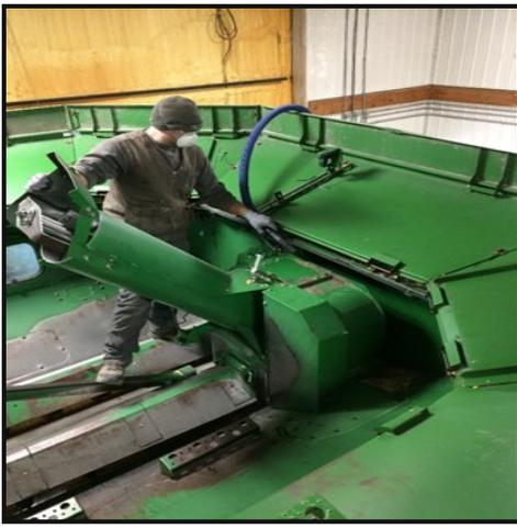
Figure 3. Vacuum the grain tank, starting from top to bottom.
