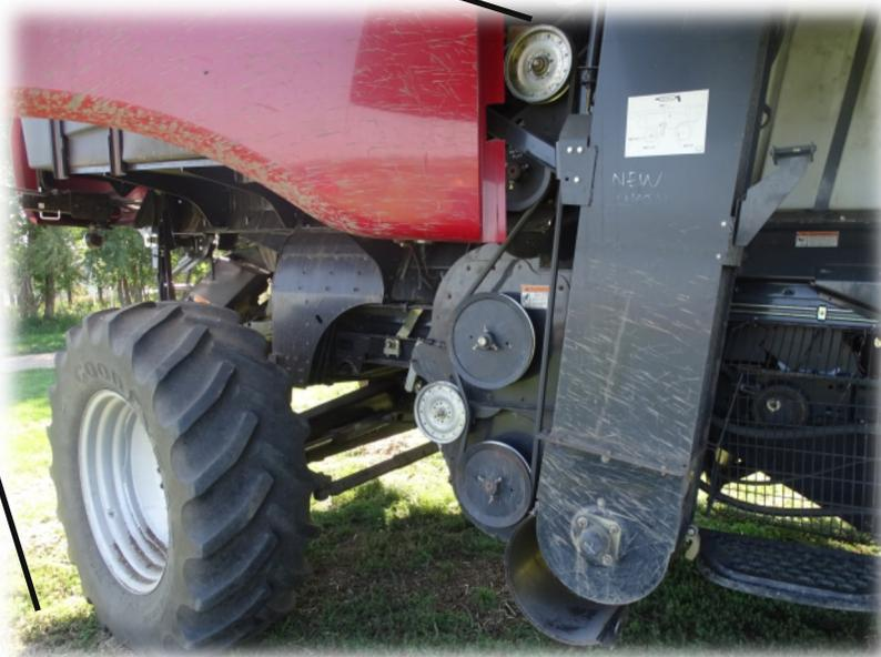
*Figure 10 (Right): Used compressed air to remove residue from the spreader assembly and rear axle of the combine.*
