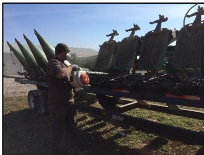
*Figure 6. Using a leaf blower to remove residue from the gathering chains, deck plates, and snapping rolls on a corn head.*
