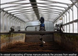
In–vessel composting of horse manure protects the process from weather An auger runs the length and width of the vessel, turning, the product. .
