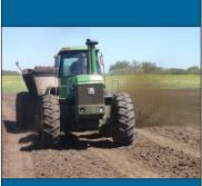
Surface applying liquid dairy manure with a side slinger manure spreader.
