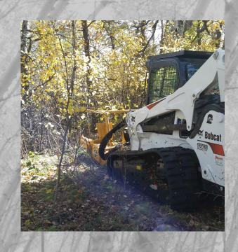
Forestry Attachment that operates by hydraulics. Disk is 60" and has cutting teeth on top, bottom, and outer edge to cut and process the materials.
