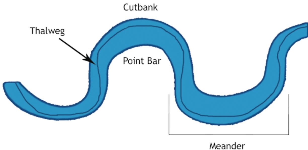
*Figure 1. Drawing of a section of a river that offers a visual representation of cut banks, point bars, and meander. The deep blue line in the river is the thalweg or deepest channel of a river, courtesy of the Cass County Soil Conservation District.*
