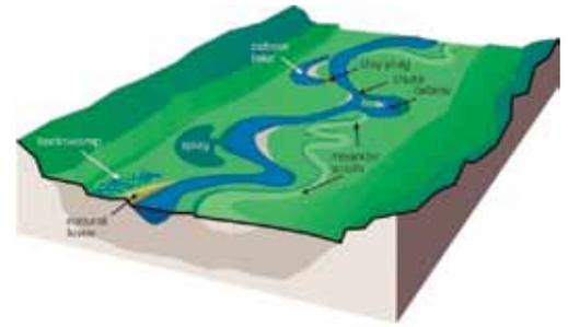
Figure 58. This illustration depicts the various landforms and deposits of a floodplain and the topographic features created by meandering streams. Adapted from "Stream Corridor Restoration: Principles, Processes, and Practices" by the FISRWG, Oct. 1998.
