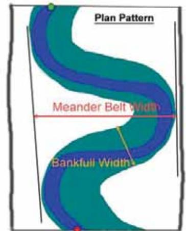
Figure 59. This illustration depicts meander belt width and bankfull width. Adapted from "Fluvial Geomorphology Module" by Endreny, 2003.
