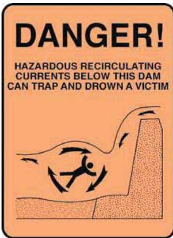
Figure 68. This is the sign posted at many dams warning of the “drowning machine” currents in “The Drowning Machine” by Elverum and Smalley and the MN DNR, 2008.
