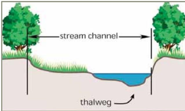
Figure 3. This cross-section drawing shows the expanse of a stream channel, the uneven bottom of a riverbed, and the thalweg. Adapted from *Stream Corridor Restoration: Principles, Processes, and Practices*, by Federal Interagency Stream Restoration Working Group (FISRWG), October 1998.
