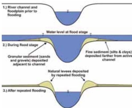
Figure 60. This diagram depicts the process of natural levee formation. Adapted from "Should I Trust that Levee?" by Rogers, 2007.
