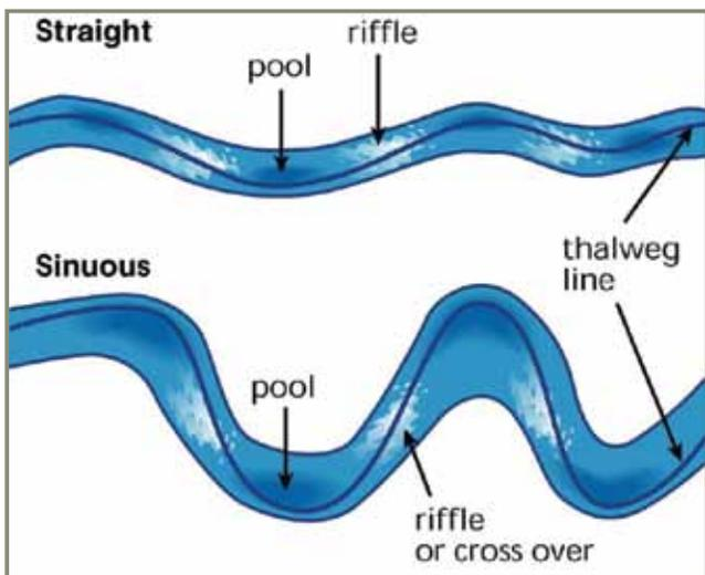
Figure 4. An illustration of sequence of pools and riffles in straight (top) and sinuous (bottom) streams. Adapted from *Stream Corridor Restoration: Principles, Processes, and Practices* by FISRWG, Oct. 1998.
