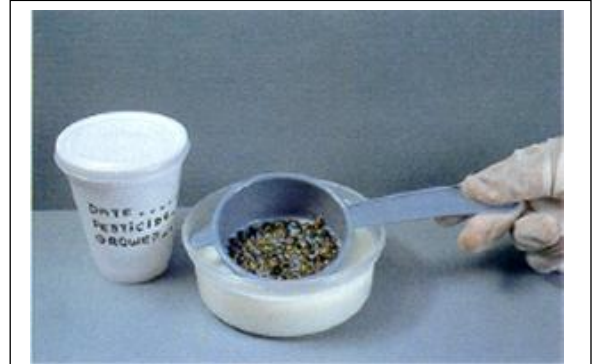
Figure 6. Dip test to determine insecticide efficacy.
