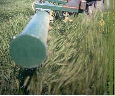
Test results indicate air assist sprayers provide good head coverage.
