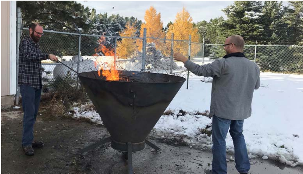
ND Forest Service staff load invasive buckthorn into the first biochar kiln fabricated to produce charcoal to be used as a soil amendment.
