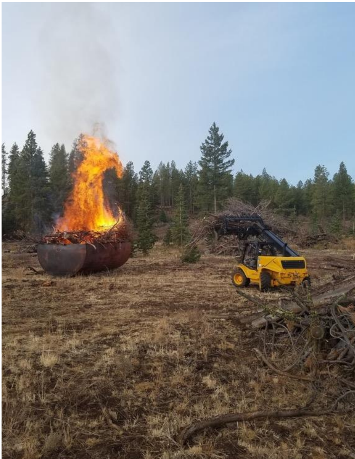
Figure 3. Arborist Brandon Baron makes biochar in a modified 10,000-gallon water tank (Photo courtesy of The Tree Service, Burns, Oregon)
