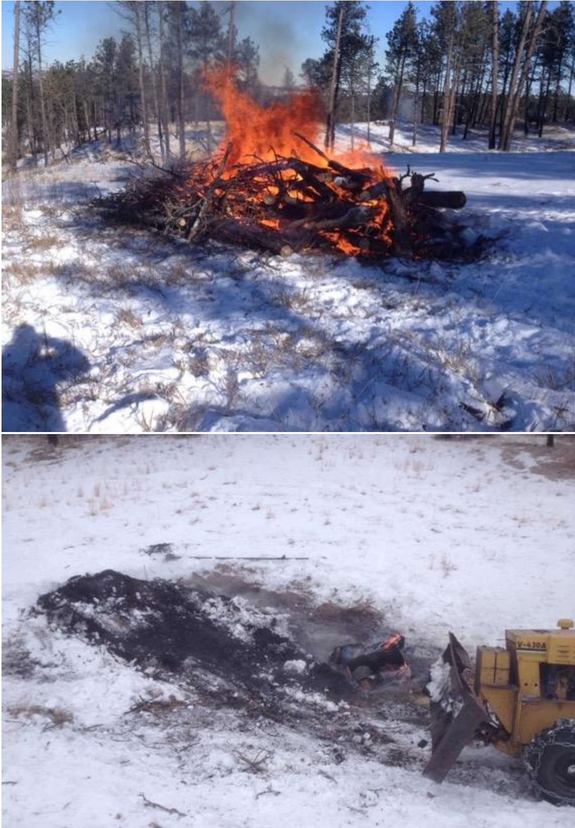
Figure 2. Snow quenching in Nebraska. Rowdy Yeatts of High Plains Biochar uses snow to quench Conservation Burn piles. Photo Courtesy of Rowdy Yeatts/High Plains Biochar, Chadron, NE.
