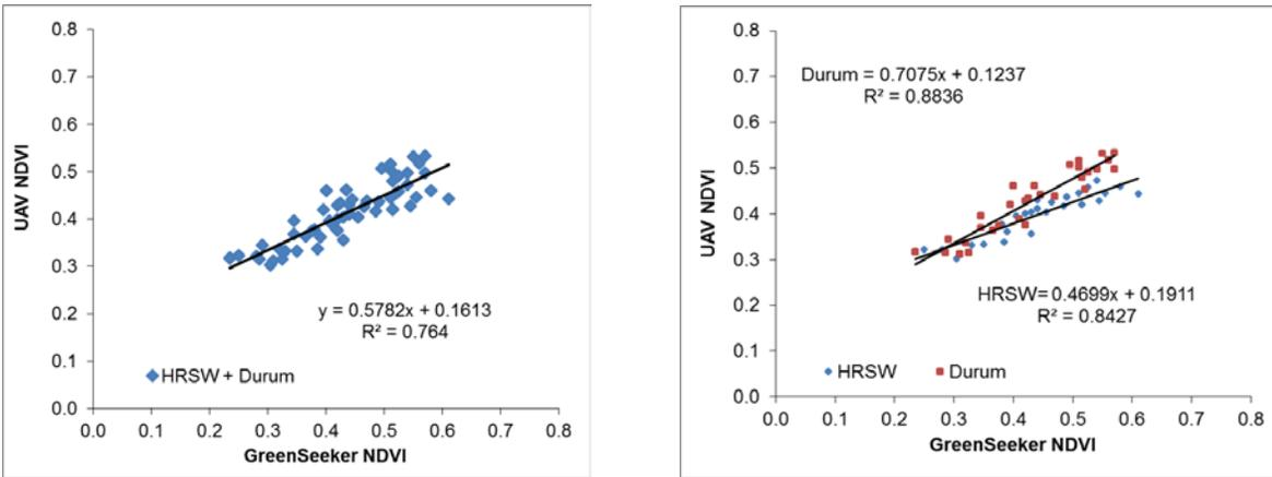
**Figure 1. UAV and GreenSeeker NDVI value correlations for hard red spring wheat (HRSW) and durum.**
