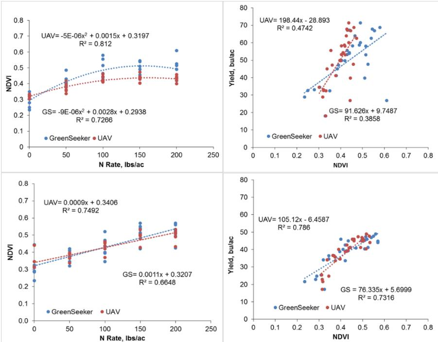
**Figure 2. UAV and Greenseeker NDVI correlation with N application rates (left) and yield (right) for HRSW (top) and durum (bottom).**
