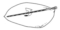
Figure 2. Recommended method of probing bags of seed.
