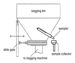
Figure 5. Automatic sampler installed in bagging bin.
