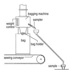
Figure 6. Automatic sampler installed in bagging machine.
