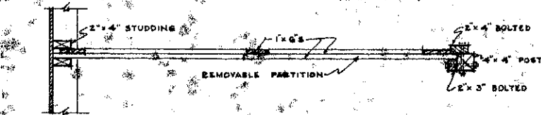
PLAN OF MOVABLE PEN PARTITION SCALE: \frac{3}{4} " = 1'-0"
