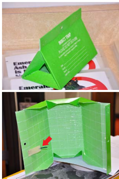
Figure 4: (Top) Assembled gypsy moth trap and (bottom) the new filmlike lure with an attachment system (red arrow) devised by forest health intern, Alec Miller (A. Bergdahl, NDFS).
