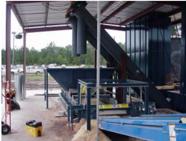
CHALLENGER ® CH500-40150-SR "Horizontal" Grinder Processes Hogged Hardwood Material to Fine Core Material
