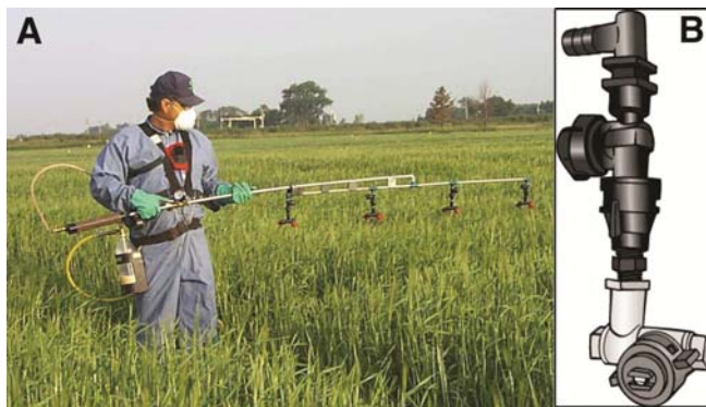
Fig. 6. A, Hand-held sprayer used for research studies with various nozzle configurations, forward/backward XR8001 flat fan illustrated, 276 kPa (40 psi), 168 liters/ha (18 gpa) at ~6.4 km/h (4 mph) (41,42,93). B, For commercial ground application of fungicides with a tractor-mounted sprayer at 16 km/h (10 mph) and 94 liters/ha (10 gpa), a single forward nozzle gives almost as much coverage and disease control as forward/backward nozzles used at slower speeds. The nozzle illustrated is a forward flat fan nozzle angled toward the grain head using a single swivel nozzle adapter (42).
