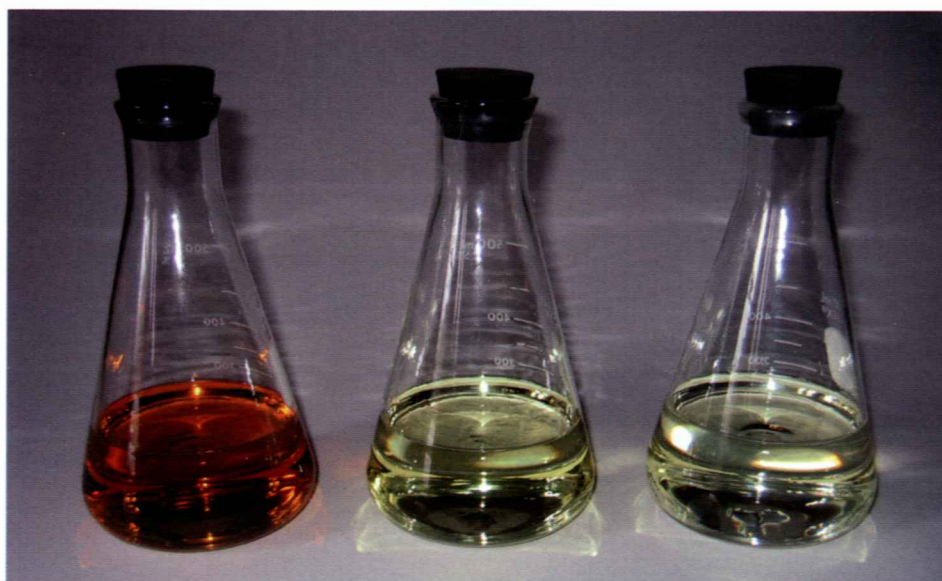
One hundred percent biodiesel (B100), center, and 100 percent soybean oil, right, are similar in color but very different in viscosity. Both differ in color from No. 2 diesel fuel, left.
