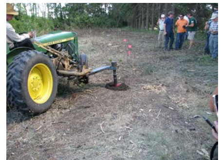
A planting hole is drilled among stumps with a modified Tre-Ro-Weeder
