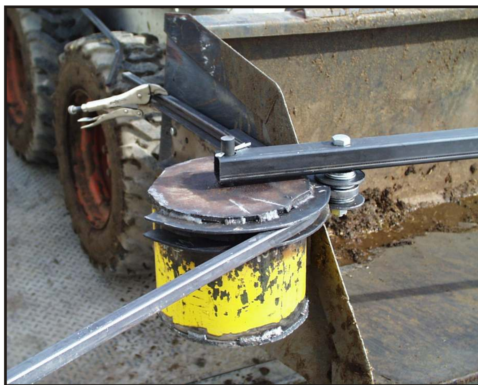
Figure 3. The hoops are formed from 3/4" square tubing shaped in a shop made tubing bender.
