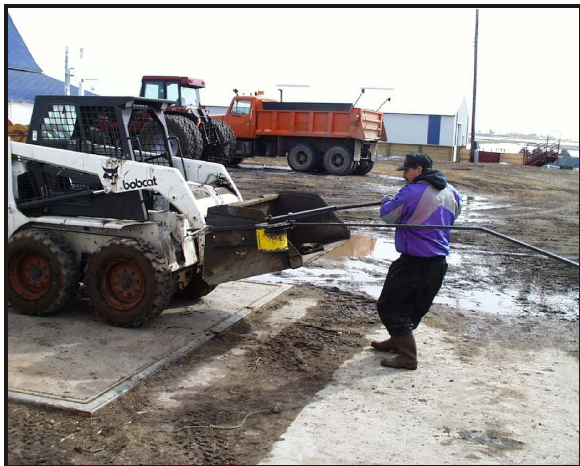
Figure 4. Fastening the tubing bender to the bucket of the Bobcat allows the work to be done at a comfortable height.
