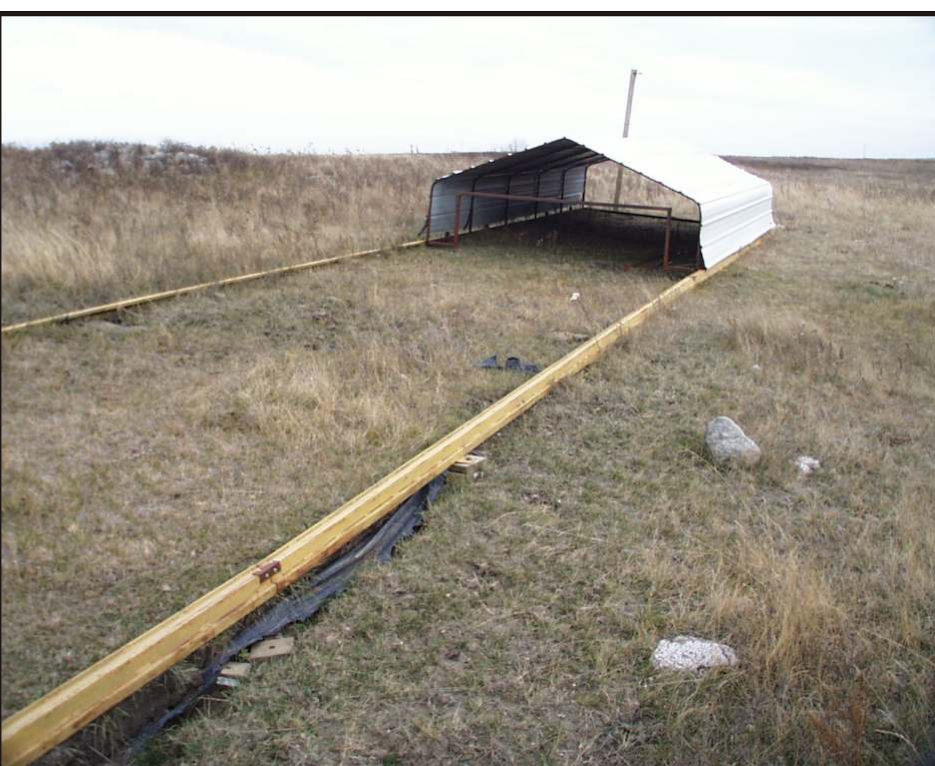
Figure 8. The cage in the open position shows the distance from the research plot. The plastic along the track was trenched to a depth of 2 feet to prevent any lateral groundwater flow. The tracks have been redesigned since
