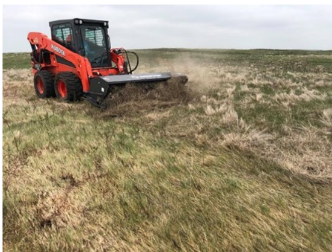
Figure 2a. 82-inch Titan Implement X-treme Skid-Steer Angle Broom Attachment connected to a SSV75 Kubota Skid-Steer.
