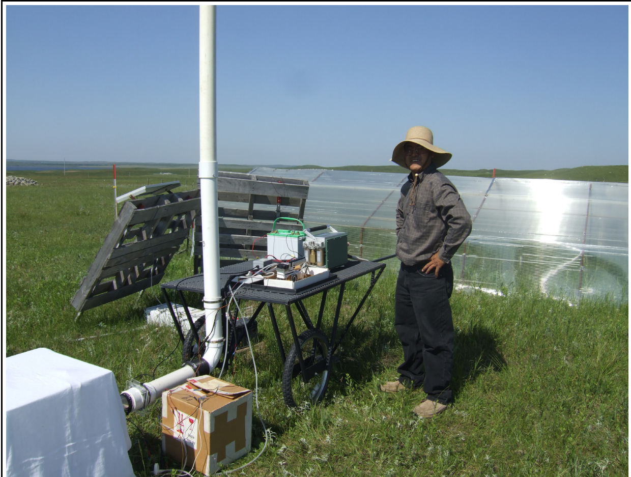
Figure 2. A transparent chamber and a gas exchange system were used to measure canopy photosynthesis from rangelands under different intensities of grazing. Various layers of cloth blankets were used to reduce light levels in order to calculate photosynthesis–light response curves.
